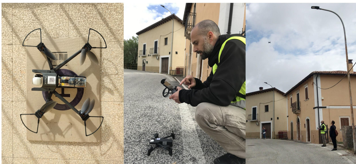
Figure 5. Parrot Anafi. Drone used for the Castelvecchio Calvisio mission. Wide-angle f/2.4 ASPH lens, 35 mm equivalent focal length: 23-69 mm (sensor set in photo shooting mode), 26-78 mm (sensor set in video shooting mode) (© S. Giraudeau, Y. A. Mazurek).
