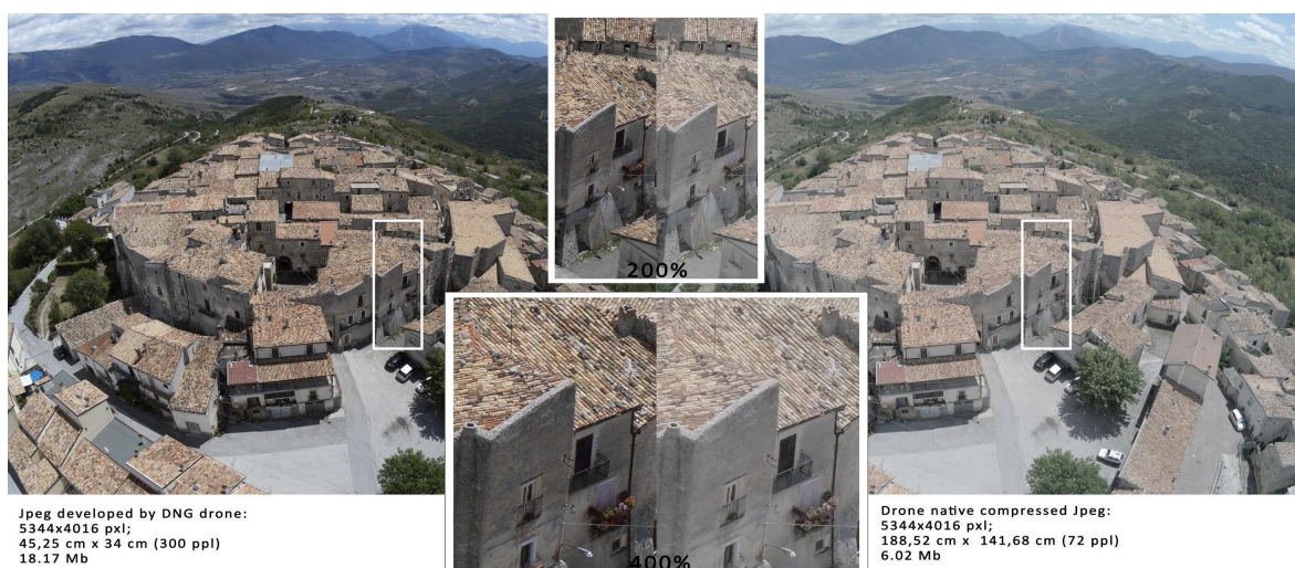
Figure 6. Comparison of the two types of JPEG files from the drone. Aerial view of Castelvecchio Calvisio, July 2020 (© S. Giraudeau).
