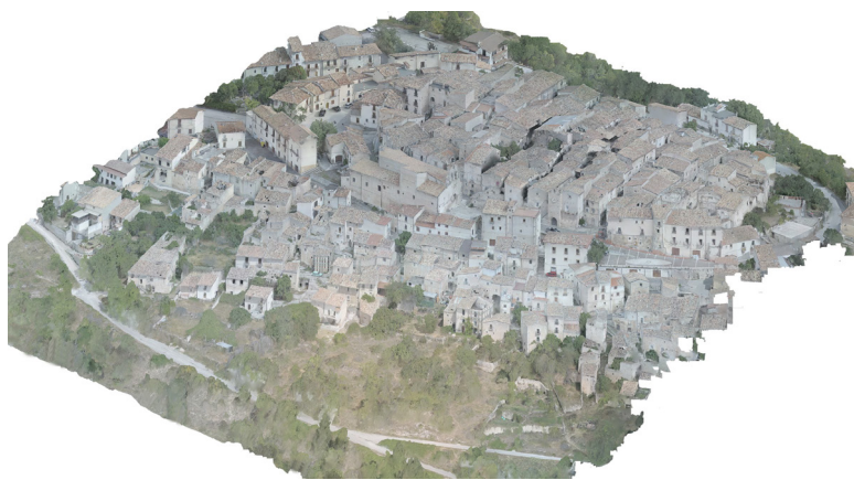
Figure 10. Aerial survey result, developed with Agisoft Metashape; 35.389.799 Faces; 17.727.890 Vertices (© S. Giraudeau, A. Leonardi, G. Verdiani).
